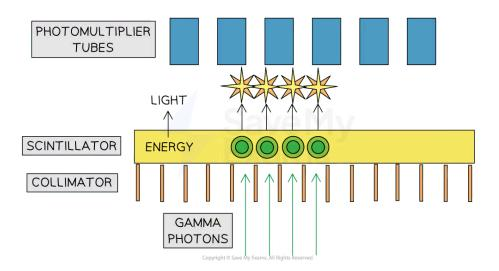
The scintillator crystal converts the energy from gamma photons into visible light photons
