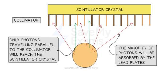
The collimator ensures high resolution images are produced by only allowing photons travelling parallel to the lead plates to pass through
