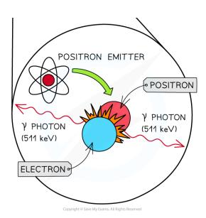
Annihilation of a positron and an electron is the basis of PET Scanning
