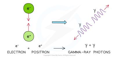
Annihilation of a positron and electron to form two gamma-ray photons
