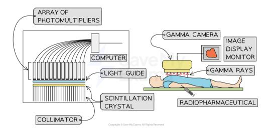
A gamma camera detects the gamma rays emitted by a radioactive tracer in the body using a large scintillator crystal connected to an array of photomultipliers
