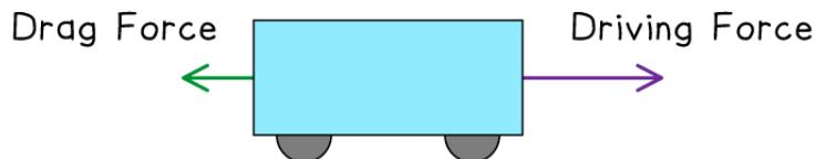
**Constant velocity****Driving force = Drag Force**
