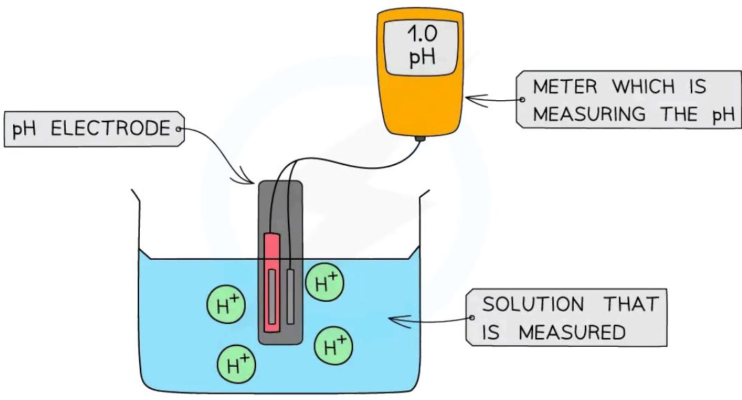
The diagram shows a digital pH meter that measures the pH of a solution using a pH electrode
