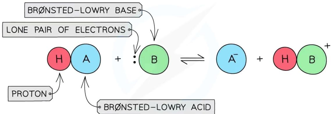
The diagram shows a Brønsted-Lowry acid which donates the proton to the Brønsted-Lowry base that accepts the proton using its lone pair of electrons
