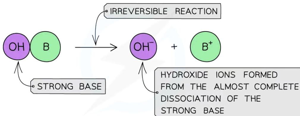
The diagram shows the complete dissociation of a strong base in aqueous solution
