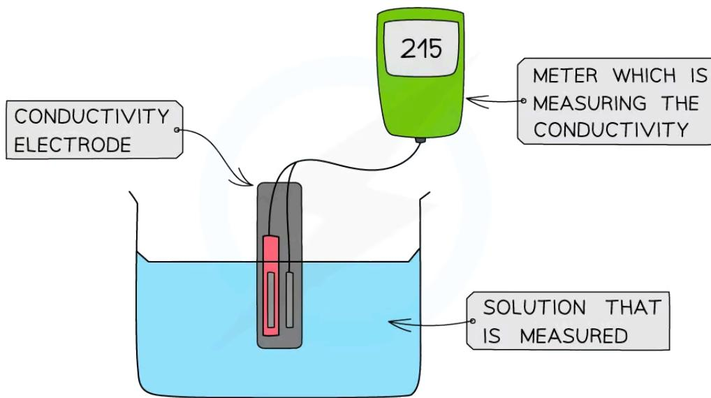
**A digital conductivity meter measures the electrical conductivity of a solution using an electrode**
