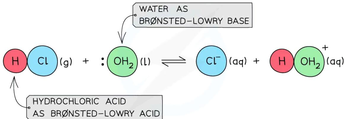
The diagram shows water acting as a Brønsted-Lowry base by accepting a proton from hydrochloric acid proton using its lone pair of electrons
