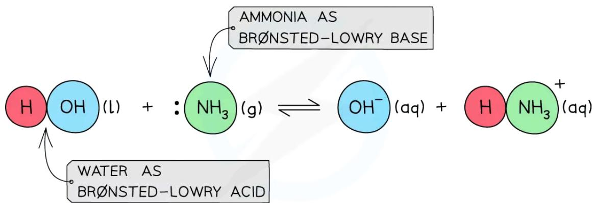
The diagram shows water acting as a Brønsted-Lowry acid by donating a proton to ammonia which accepts the proton using its lone pair of electrons
