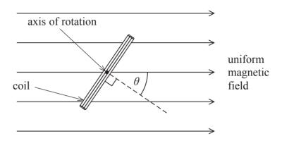
(a) The coil has 200 turns and an area of  $2.0 \times 10^{-4}$  m<sup>2</sup>.
