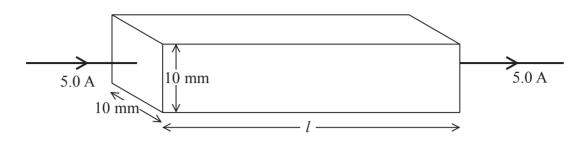
The bar is placed in a magnetic field so that its weight is supported by the magnetic field.
