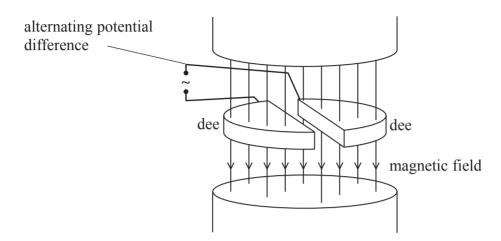
With reference to the magnetic field and the alternating potential difference explain how the cyclotron produces a beam of high speed particles.
