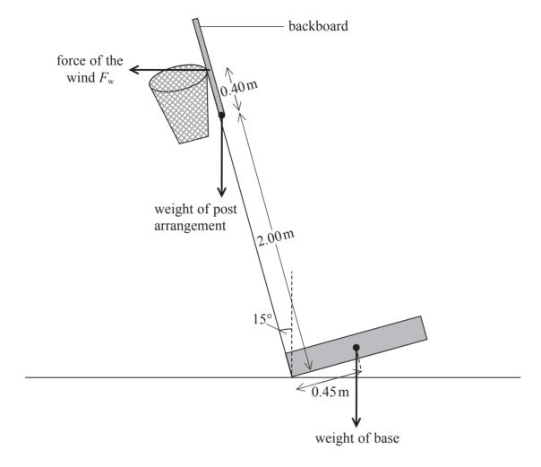
Calculate the minimum force of the wind  $F_{\rm w}$  that will cause the basketball set to be blown over when it is at the angle shown. Ignore the effect of the wind on the base.
