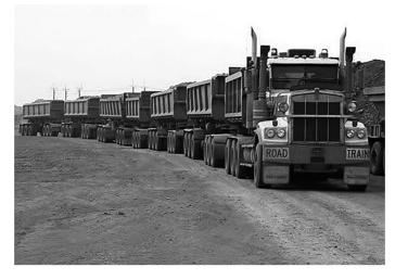
(a) The braking distance of a road train travelling at 15 m s<sup>-1</sup> is 70 m.
