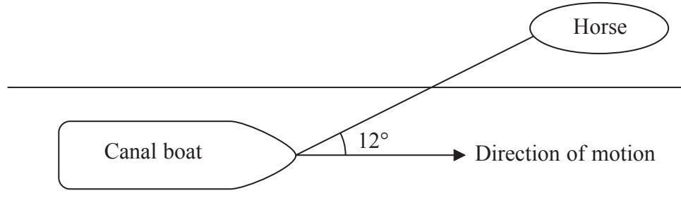
A horse is pulling a canal boat using a rope at  $12^\circ$  to the direction of motion of the boat. The tension in the rope is 1150 N.
