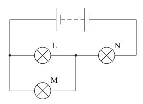
The filament of lamp M breaks. Identify the row of the table which shows the resulting changes in the brightness of lamps L and N.
