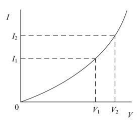
Which row of the table gives the resistance of the component at  $V_2$  and describes how the resistance changes from  $V_1$  to  $V_2$ ?
