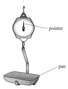
When vegetables are added to the pan, the weight of the vegetables causes a spring to extend, moving the pointer on the scale.
