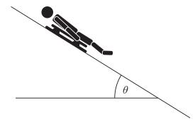
Draw a free-body force diagram for the sledge and athlete. You should consider the relative sizes of the forces when drawing your diagram.
