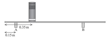
(a) The normal contact forces of each bracket on the shelf are equal.
