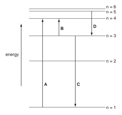
23. The diagram shows part of a simplified emission spectrum of hydrogen.
