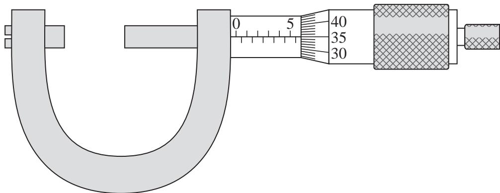
Which is the correct reading of the gauge in millimetres?
