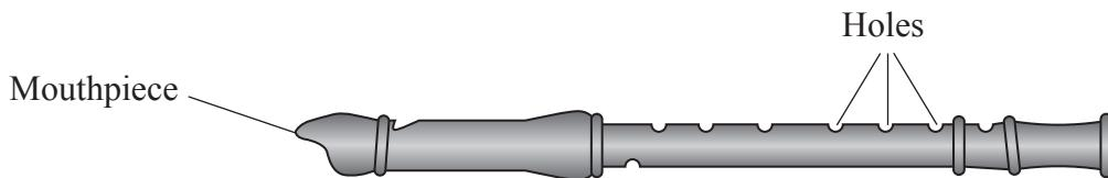
The length  $l$  of the vibrating air column is changed by covering the holes. This changes the frequency  $f$  of the sound produced.
